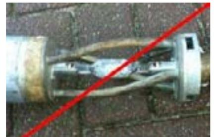
**The light source must always be tested to make sure it is in good working order before it is brought into the pipe.**
