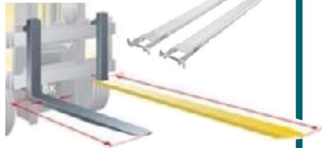
When transporting and lifting crates with a forklift truck, make sure the forks are always supporting the entire width of the crate. If the length of the forks is less than the crate width, there is a risk, when the crate is lifted, nails will be pulled out of the crate resulting in damage to the crate or material inside. Appropriately dimensioned fork extensions (as shown in the image) must be used.
